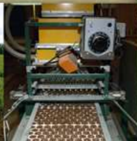
Automated multi-pol filling and seeding line
