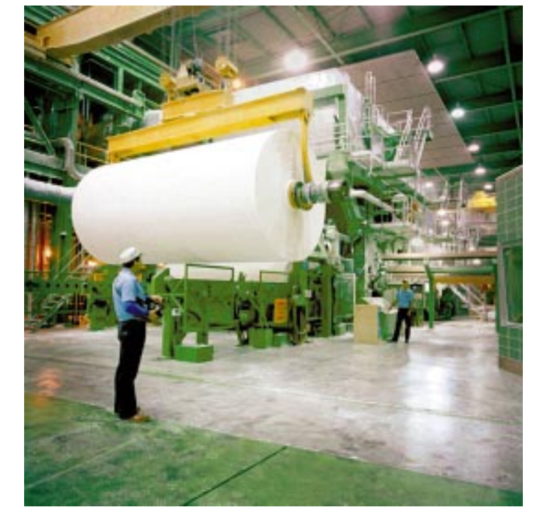
Transferring Roll to Winder - Overhead Crane
